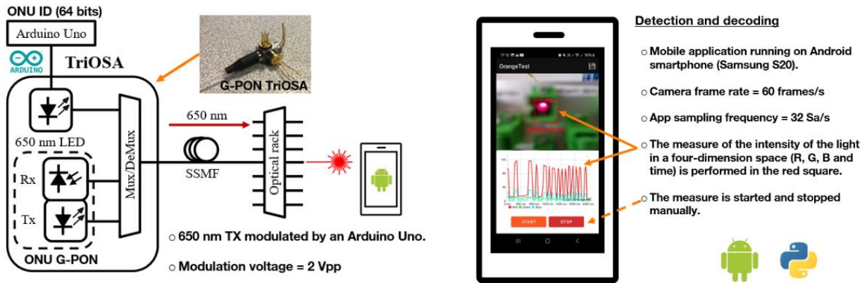
Figure 29: Integrated TriOSA carrying ONU ID and read-out on smartphone app
