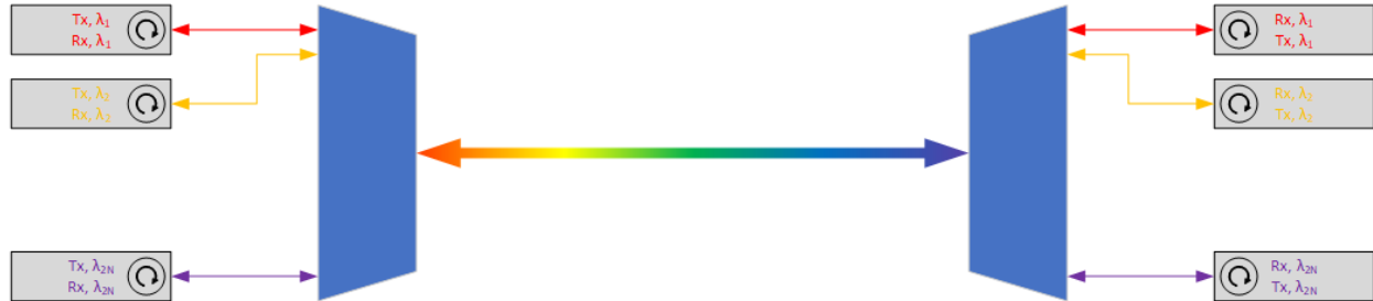
Figure 2 Single fiber DWDM link using bidirectional DCO transceivers with optical circulator.
