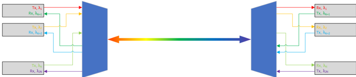
Figure 1 Single fiber DWDM link with separated wavelengths for upstream and downstream traffic.
