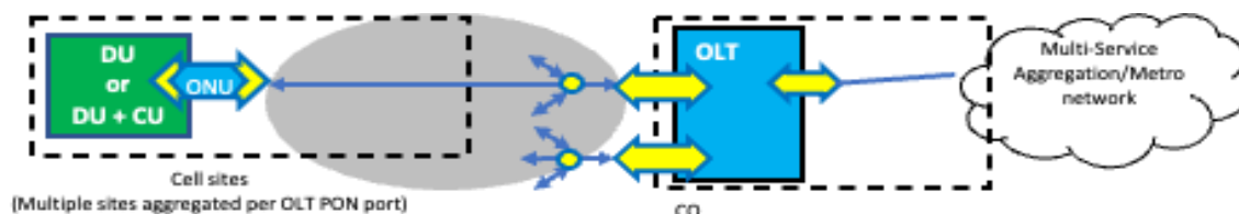
Figure 33: Up to 20 km backhaul and HLS with TDM-PON using pluggable ONU. HLS is depicted in cases where the CU is centralized. Backhaul is depicted in cases where the CU is located at cell site.
